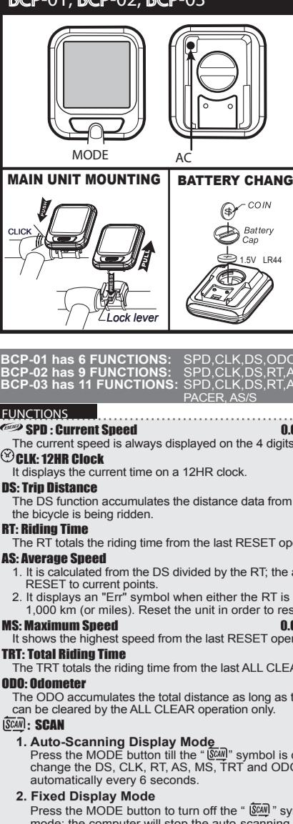
Fig.1 Main unit setup
