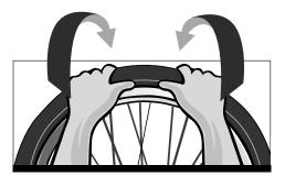
5. Check while moving the tire from the front to the rear if the inner tube is completely inside the tube.
