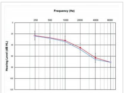
Figure 1. Average hearing level thresholds for right (red) and left (blue) ears of all participants. Error bars show one standard deviation for the right ears. Standard deviation for the left ears was nearly identical and omitted here for
