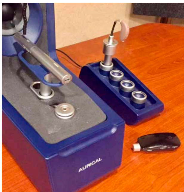
Figure 2. For validation of the adaptive gain using the ReSound Multi Mic, the Roger Pen microphone was placed inside the HIT box, and the Roger X universal was plugged into the ReSound Multi Mic. The ReSound Multi Mic was placed outside the HIT box and set up to stream to the ReSound LiNX 2 hearing aid, which was mounted on the external coupler for measurement.
