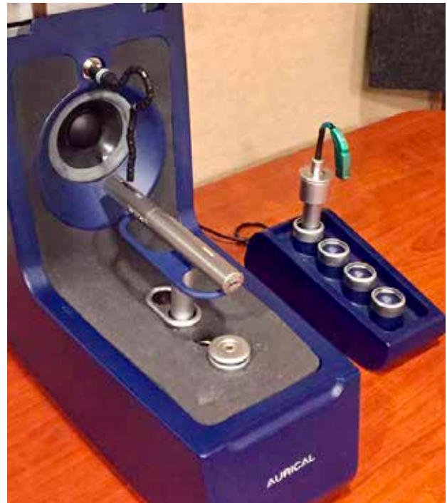
Figure 1. For validation of the adaptive gain, the Roger Pen microphone was placed inside the HIT box and the Phonak Sky hearing aid was mounted on the external coupler for measurement.
