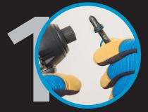
Choose bit size & attach it to the chuck or coupler. Fasten it well. Set the power tool to MAX speed & torque if it is adjustable. Wear eye, face protection, and gloves.
