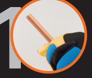
Firmly hold tubing at all times. Keep a safe distance between your hand and the tube's border. Wear eye, face protection and gloves.
