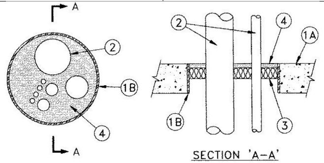
1A. **Floor or Wall Assembly** — Min 2-1/2 in (64 mm) thick floor or 3 in. (76 mm) thick wall of reinforced light weight or normal weight (100-150 pcf or 1600-2400 kg/m³) concrete. Wall may also be constructed of any UL Classified **Concrete Blocks**\*. Max diam of opening is 15-1/4 in. (387 mm).
