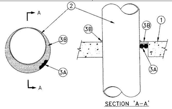
1. Floor or Wall Assembly — Min 2-1/2 in. (64 mm) thick reinforced light weight or normal weight (100-150 pcf or 1600-2400 kg/m³) concrete. Floor may also be constructed of any 6 in. thick UL Classified hollow-core Precast Concrete Units\*. Wall may also be constructed of any UL Classified Concrete Blocks\*. Max diam of opening is 24-7/8 in. (632 mm). When precast concrete units are used the max diam of opening is 7 in. (178 mm).
