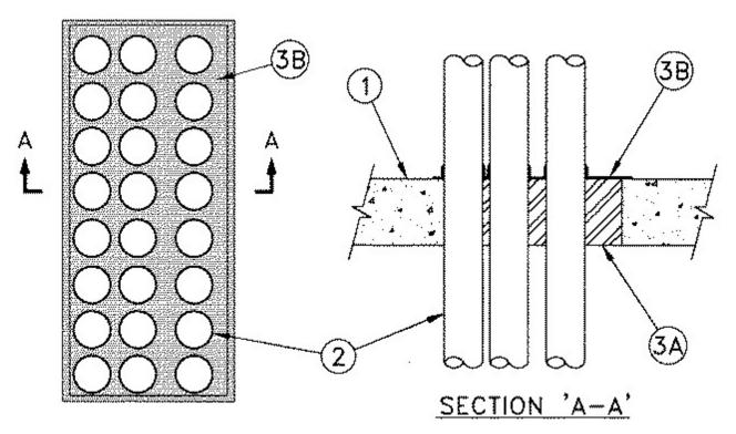
1. Floor or Wall Assembly — Min 4-1/2 in. (114 mm) thick reinforced light weight or normal weight (100-150 pcf or 1600-2400 kg/m<sup>3</sup>) concrete. Wall may also be constructed of any UL Classified Concrete Blocks\*. Max area of opening is 864 sq. in. (0.56 m<sup>2</sup>) with max dimension of 48 in. (1.22 m).
